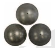
Nickel Bonded Diamond Domes are an excellent choice for working bottles and inside curves. These domes are approximately 3-7/8" at base and 1-1/2" in height. Standard sizes available are: 1"-14 female and 5/8"-11 female. Cones are available in Coarse (100g), Medium (220g), and Fine (600g). All domes include a 3/16" center hole for through-shaft water systems.
