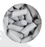
Ceramic Angle #2 contains a mild abrasive. An excellent filler, it adds weight to the load increasing tumbling action, separates work pieces keeping parts from sticking together, and carries grit to work pieces.
