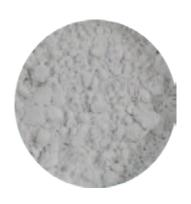
This 98% pure levigated alumina polish powder is excellent for tumbling, pre-polishing, and plate lapping.
