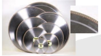
Covington's Platinum Series 301 Lapidary Blades are made with a higher diamond concentration and a higher carbon content steel core for improved tension memory. The solid diamond sintered kerf provides better cutting performance and improved coolant flow. Covington's Platinum 301 is an excellent choice for cutting hard materials such as agate, petrified wood, or jade. \*Please specify arbor size when ordering.
