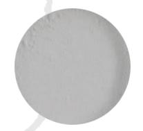
A 99% pure micro alumina powder, this polish is excellent for achieving a super-fine polish on all hard and soft stones. Particle size is approximately .5 microns and a 9 on the Mohs scale (compares with Linde 'A' Polish).
