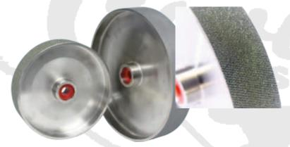
Covington's 6" and 8" Textured Grinding Wheels are excellent tools for pre-forming rough stone and glass material. The texturing allows for better sediment wash-out. These balanced, solid steel wheels, are nickel electroplated to provide superior bonding of diamonds and a long life.
