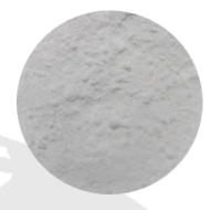
A .3 micron alumina powder that is 99.98% pure aluminum oxide and a 9 on the Mohs scale. Linde 'A' will polish almost any gemstone.
