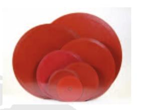
Sintered Diamond Blades are a longer lasting blade compared to the notched rim. These blades are manufactured by embedding diamond grit directly into the metal matrix that forms the edge of the saw blade. Sintered blades are a better value than other blades because of their long life.
