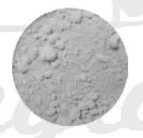
This 99.9% high purity tin oxide provides an excellent polish on almost any gemstone including hard-to-polish stones.
