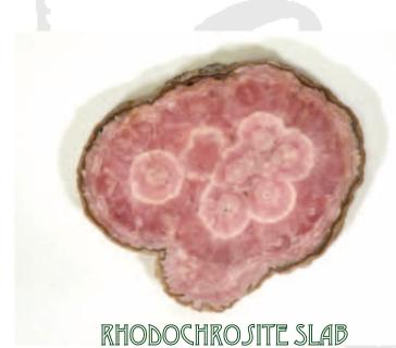
This Rhodochrosite slab was cut on a Covington Slab Saw. This 1/4" slab was cut from a 4" rock using the 16"Covington Combination Slab Saw (1172CS). It was then ground and polished on a Flat Lap Unit. Read about our flat laps on page 42.
