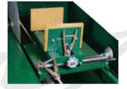
This book-end type vise holds work pieces of any shape tightly, but quick-release feature allows an easy, no-bind return. The steel jaw tongue contacts the full length of the vise, holding the jaw square so it can't bind. The end grips have a hardwood facing. A cross shaft is included with each vise.
