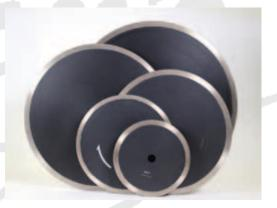
Sintered Diamond Blades are a longer lasting blade compared to the notched rim. These blades are manufactured by embedding diamond grit directly into the metal matrix that forms the edge of the saw blade. Sintered blades are a better value than other blades because of their long life.
