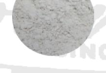
Use on cork belts, wheels, or discs for semi-polishing the edges or bevels on glass plate. This pumice creates an excellent pre-polish on glass.
