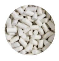
Ceramic Angle #3: This filler media adds weight to the load effectively increasing tumbling action, separates work pieces keeping parts from sticking together, and carries grit to work pieces.
