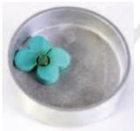
The Putty Vise holds small pieces of gemstone or glass for drilling. Always drill with the work piece submerged in water to keep the drill bit cool and to sustain a longer drill bit life. This unit comes with a 3" diameter x 5/8" deep aluminum tank, a 1" square block of plastic putty and a 1/4" brass ferrule. The plastic putty holds the work piece and the brass ferrule can act as a dam to hold grit or water when drilling.
