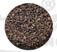
An excellent aid to grinding and polishing in a vibrating or rolling tumbler. The small size aids in reaching hard-to-get areas. Use 1/4- cup of garnet sand per quart of rocks. Use the mixture from rough grind through polish. 8/12 mesh.
