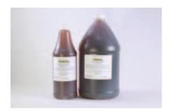
Covington's #2 Koolerant is designed for cutting large pieces of hard or dense rock. This Koolerant is an excellent choice for cutting any size rock that requires a high heat factor at blade contact because of the raised flashpoint. Add 9 parts of light form oil (Rock Hound Oil, mineral oil, etc.) to each part of Covington's concentrated diamond blade Koolerant #2. Mix well before pouring into the saw.
