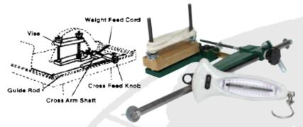
The Trim Saw Vise and Cross Feed are designed to slab small work samples. The vise jaws hold up to a 3-1/2" rock and grip the work piece without blocks or shims. The cross feed adjusts 3-1/2" before repositioning the stone in the vise. The end of the cross arm shaft has a "no bind" roller bearing and hook which ensures a smooth feed and prevents rocks from "riding up" the blade. This kit comes complete with a vise assembly, cross arm shaft, cross feed, knob, weight feed cord, and scales.
